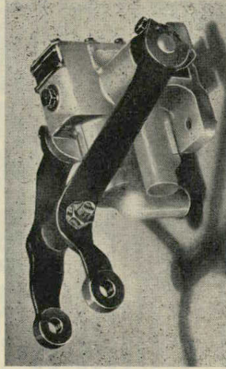
ARMSTRONG TUBULAR AIRCRAFT TYPE. A PARTICULARLY EFFICIENT UNIT EQUIPPING MANY ENGLISH AND AMERICAN CARS AND BUSES WITH CONVENTIONAL SPRINGING.
